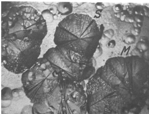
Figure 2 An example of single (marked S) and multiple (marked M) nucleation centres for growth of hillocks. Etching time 4 h, temperature 21° C ( \times 126 ).
